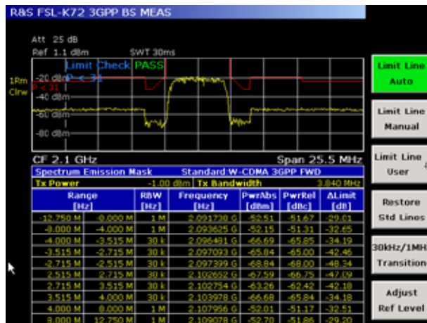
The spectrum emission mask measurement is defined with a 30 kHz measurement bandwidth at 2.5 MHz to 3.5 MHz offset from the carrier. From 3.5 MHz to 12.5 MHz, the measurement is performed in a 1 MHz measurement bandwidth. The limit values are in line with 3GPP specifications TS 25.141
